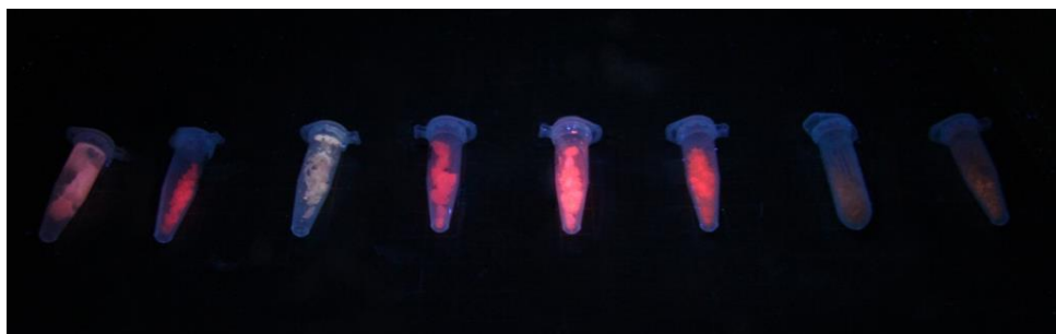
Figure 1. Multicolor emission in Eu 3+ -doped silicates.
