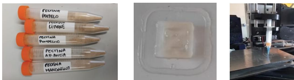
Figure 1. Different samples of pectin from different citrus fruits on the left, 3d printing test in the middle, 3D extrusion printer on the right.
