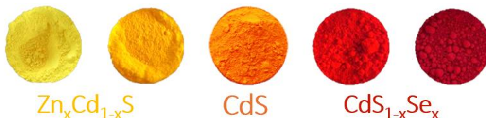
Figure 1. Chromatic variations of cadmium-based pigments: yellow ( \text{Zn}_x\text{Cd}_{1-x}\text{S} ), orange ( \text{CdS} ), and red ( \text{CdS}_{1-x}\text{Se}_x )
